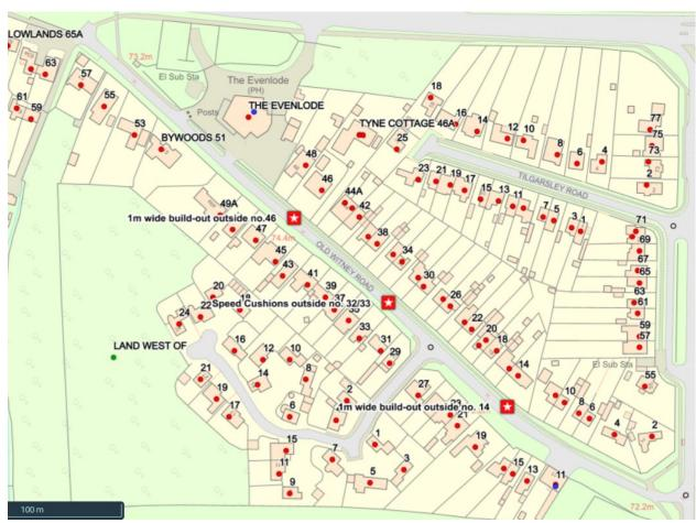
Calming features include build-outs with priority signing and speed cushions which aim to slow traffic without interfering with emergency vehicles.
