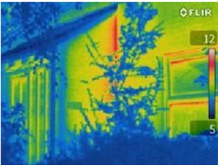
A thermal image showing heat loss around a window frame. The image is color-coded, with red and yellow indicating high heat loss and blue indicating low heat loss. The window frame and the area around it are shown in red and yellow, indicating significant heat loss. The text 'FLIR' is visible in the top right corner of the image. A temperature scale on the right side of the image shows values from 5 to 12.
