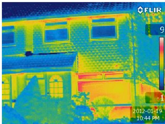
*Radiator heat loss - front wall*
